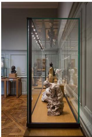
**Photo 3:** All the showcases in the museum are equipped with LED MICROTOOLS modules that can be tilted (flood beam, 4000 K). The lighting intensity can vary from 1% to 35% depending on the daylight situation.
