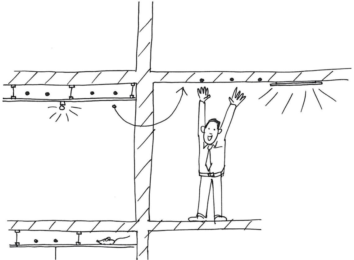
B5 | Lower buildings thanks to omission of suspended ceilings and false floors, and consequently lower construction costs.
