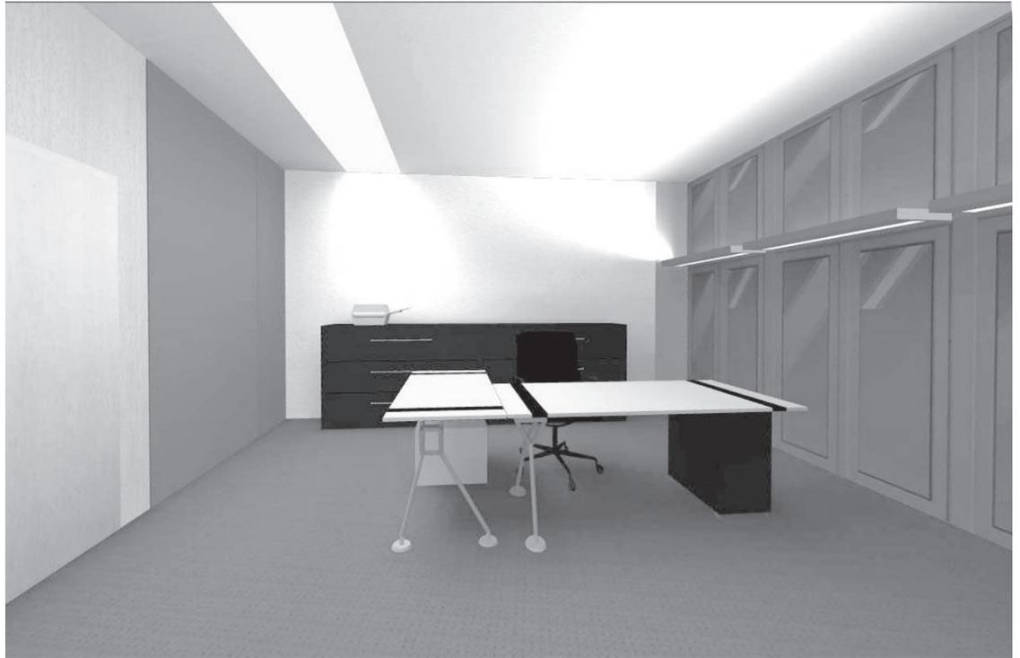
B3 | Room lighting concept: Two components ensure appropriate ambient illuminance across the entire office area: a luminaire integrated into the façade, which radiates light indirectly via the ceiling and into the direction from which daylight is entering, and a flat wide-area luminaire („artificial skylight“) with direct distribution located in the depth of the room.
